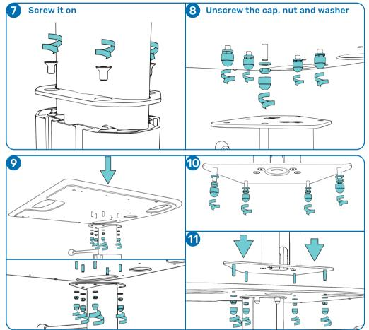
We are using a rail in the column to fix accessories. Mind the order of the accessories before fixing them!
